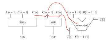
In an arithmetic logic unit (ALU), one may share the same ADDER(n) for signed addition and unsigned addition.
